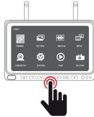
3. The monitor shows the pairing procedure via "countdown" on the screen
