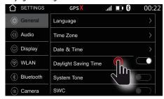
The slider next to **Daylight Saving Time** activates the daylight saving time display and the current time is advanced by 1 hour.
