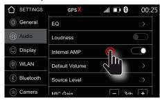
Under Internal AMP you can switch the device's integrated audio amplifier on or off. If you are using the device's preamp outputs to drive an external audio amplifier, turn off the amplifier.
