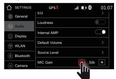
Under **Microphone Level** you can adjust the volume of the handsfree microphone with -/+.
