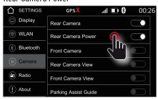
Here you can switch on the rear or front camera, switch on the respective power supply via the device and activate the respective view in the camera menu.
