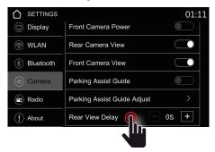
The **Rear Camera Delay** function increases the time it takes for the reverse gear vision. Settings range from 0 to 2 seconds.
