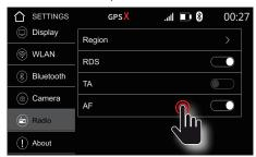
With AF, the radio switches to an alternative, better frequency of the station in the network if the reception signal is too weak and an alternative frequency is available.
