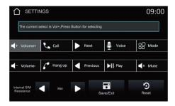
To pair, perform a function reset. Then press the first function you wish to pair (i.e., volume up) and press the corresponding button on the steering wheel.
