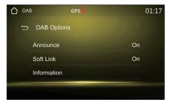
In the settings you will find the function to activate or deactivate the announcements, the Soft Link function to suppress the initial noises.
