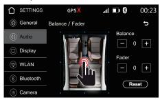
Under **Balance/Fader** you can adjust the balance of the acoustic stage between left and right and front and back.
