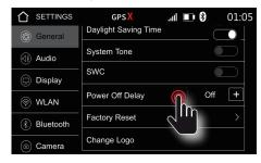
You can set a shutdown **Power Off Delay** between Off (0) and a maximum of three seconds. Use the +/- cursors to select the desired shutdown time.
