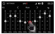
In **EQ** mode you can manually adjust the 10 audio bands available to the equalizer from -6dB to +6dB or use the  $\leftarrow$  /  $\rightarrow$  buttons to select one of the presets:
