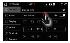
Under **Date & Time** you can set the desired time format (12H/24H) as well as the date and time manually if you want to change the time and date display determined by GPS.
