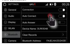
Under **Auto Connect** whether your smartphone should be automatically connected to the device after a restart.
