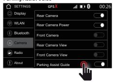
You can use the **Park Assist Guide** slider to turn on the rear view camera guidelines.
