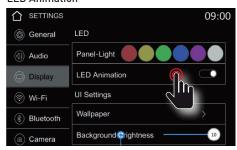
By disabling the **LED Animation** function, you can change the colors of the illumination of the front keys on the LCD panel.
