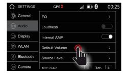
With **Default Volume** and **Source Level**, you can tune and adjust the levels for each application and signal source as desired.
