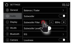
**Subwoofer** activates the SUB1/SUB2 preoutputs. The cut-off frequency can be set under the Subwoofer Filter, i.e. all frequencies above are filtered out
