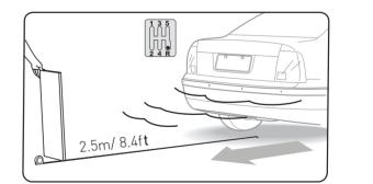
The function test is performed by holding a wooden board (0.3 m x 1 m) behind the car, go slowly in reverse to check all the functions indicated in this manual.
