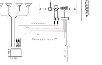
Follow the assembly and wiring instructions for the RCA audio input:
