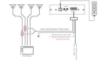
Follow the assembly and wiring instructions for the speaker audio input (high level):
