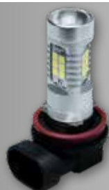
ML9330 LAMPADE LED SERIE POWER H8 12V, 5.6W, 1560 LUMEN (per kit) 6000K, 21 CHIP 2835
