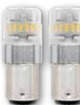
ML9390 LAMPADE LED SERIE POWER P21W 12V, 5.6W, 1560 LUMEN (per kit) 6000K, 22 CHIP 4014SMD
