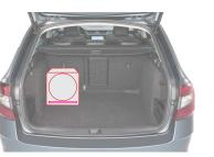
To fix the speaker we recommend using a Velcro adhesive or with the help of two metal brackets.
