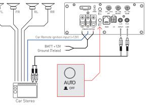
Follow the installation instructions and wiring connection to ensure the integrity of the product.
